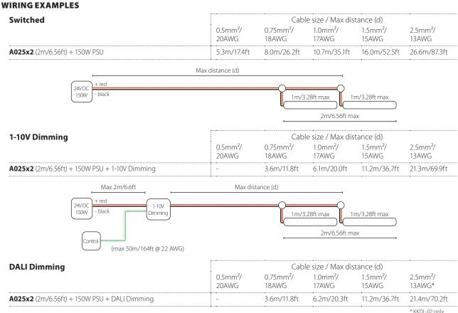
Note: This guide is produced from testing with KKDC approved power supplies or control gear.
